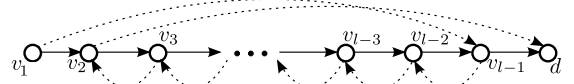
Fig. 1. Network with old (solid) and new (forwarding) rules which requires l - 2 \in \Omega(n) rounds to update consistently when enforcing loop freedom. For example, v_3 cannot update before v_2 , and so on.
